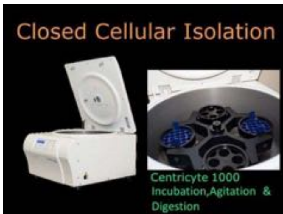
Figure 8: Centricyte 1000 (Healeon Medical, Newbury Park, CA, USA). Programmable system for isolation/concentration permitting cSVF deployment via intravenous route.
